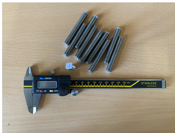
Figure 4: Bolts and calipers from Measuring bolts-puzzle . The bolts are indistinguishable by eye, and have numbers on top of them.
