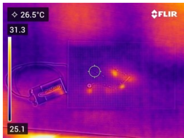
Figure 1: IR-camera picture of the Faulty Wiring -puzzle. The resistors that are used, and the LED, light up.
