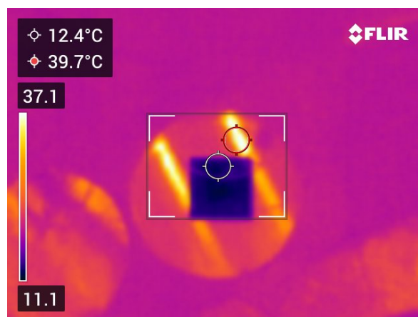
Figure 7: IR-image of a peltier element on top of a heat sink. The peltier element is shown in blue, and the heat sink is shown in orange.
